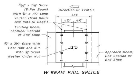
Typical Rail Splice connection detail. Source FLDOT 2014.
